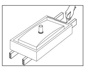
After checking fit and alignment, turn sink upside down and apply a generous portion of silicone adhesive around the under side of the rim near the edge. Place sink in position. Wipe off excess adhesive.
